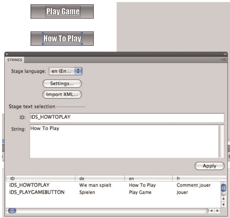
Figure B.4 Each localized text field has an associated ID to uniquely identify it.
